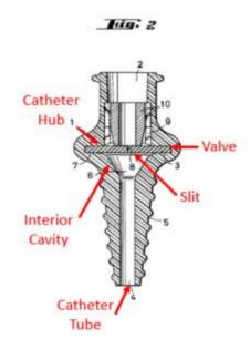
Petitioner asserts that Tauschinski discloses valve 3 with slit 8 configured to obstruct fluid flow through catheter hub 1. *Id.* at 15–16 (citing in-part Ex. 1005, 3:14–19). Petitioner reasons that it would have been obvious to modify Woehr "by adding protective elements, such as a valve to prevent the emergence of blood," as disclosed by Tauschinski. *Id.* at 17 (citing Ex. 1002 ¶¶ 63–68).
