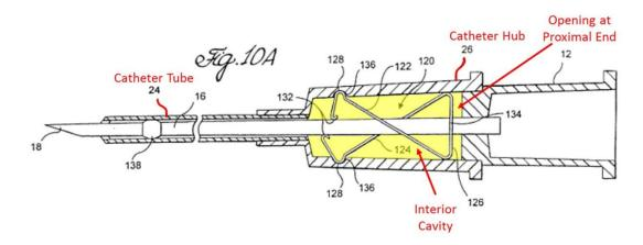
According to Petitioner, and referring to annotated Figure 10A, Woehr discloses the claimed "catheter hub" and "body," "interior cavity," (element 26) including the step of "positioning a needle protection device at least partially inside the interior cavity" (element 120). *Id*.
