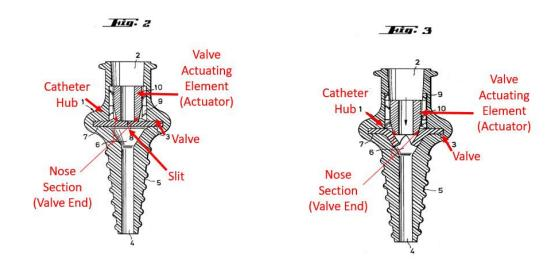
According to Petitioner, and as shown in the above Figures 2 and 3, Tauschinski discloses valve actuating element 10 slidingly disposed in catheter hub 1, and configured to actuate valve 3 to open slit 8. *Id.* at 19 (citing Ex. 1005, 3:20–36).
