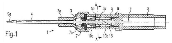
According to the '762 patent, Figure 1 depicts catheter insertion device 1 with catheter 4, needle hub 8, to which hollow needle 9 is fixed and which needle 9 passes through valve disc 7 and extends through catheter 4.
